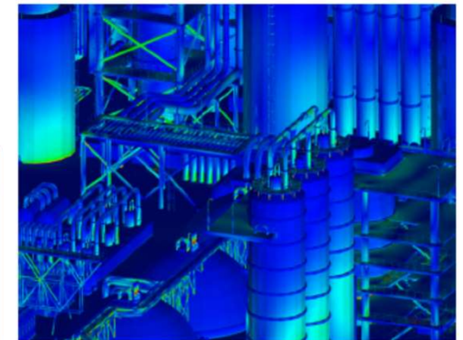
e) Stress response (von Mises-stress)
